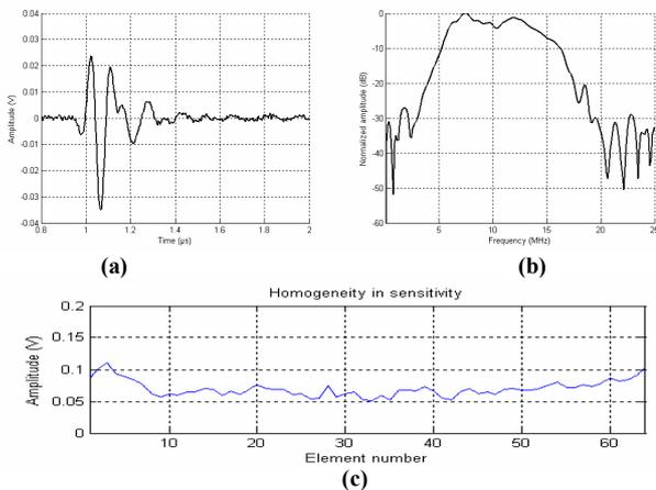
**Figure 4 : Pulse (a) and spectrum (b) response for a typical element of the transducer. Homogeneity in sensitivity (c) for all transducer**
