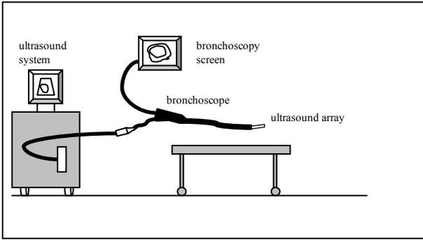
**Figure 1:** ultrasound probe is inserted through the working channel of a regular bronchofiberscope allowing combined bronchoscopy and ultrasound imaging.
