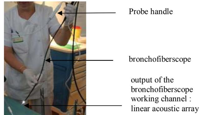
**Figure 5 : Picture of the probe inserted in the bronchofiberscope**
